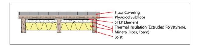
Where STEP Warmfloor® heating elements are installed on a wood subfloor, the connectors and wires can be routed under the subfloor between joists.
